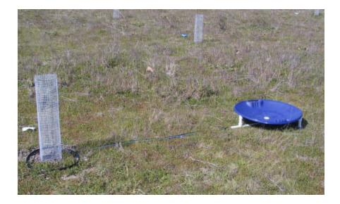
**Figure 24.** Water addition treatment. The modified disc collects and redirects additional water to oak seedlings with each rainfall event.
